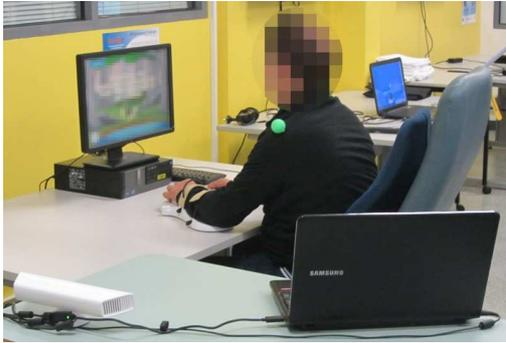
Figure 2: Subject using the system. The feedback is computed and provided by the laptop, whereas a separate VR game is run on the desktop computer.
